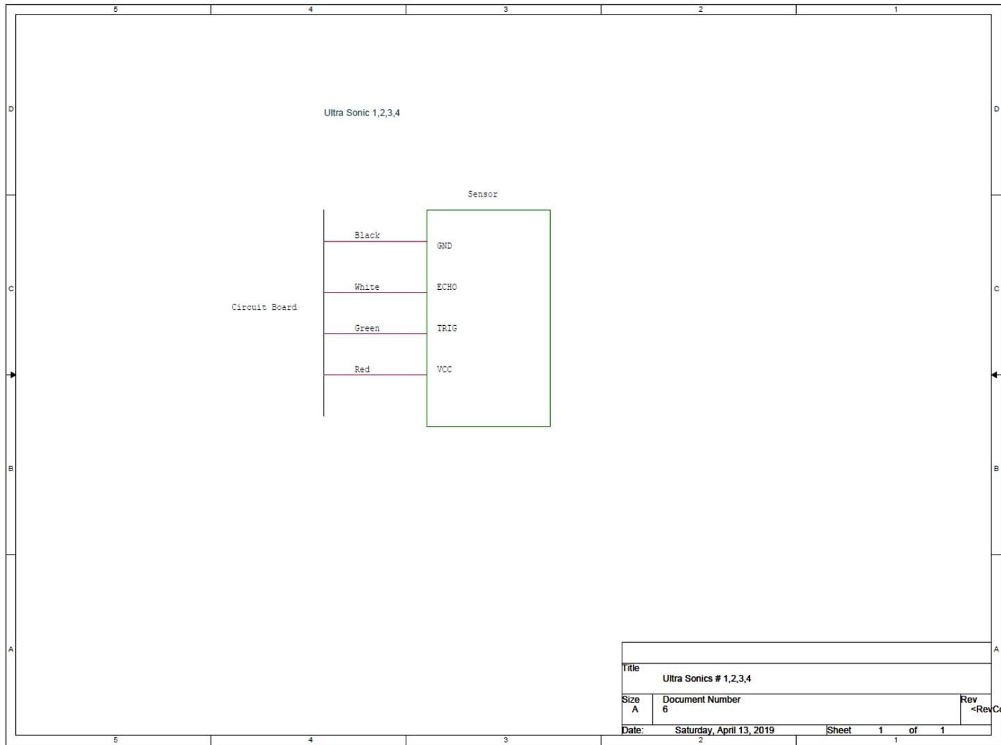
B-10. Four ultrasonic sensors are used all around, their wiring is identical among all four. A representation of their wiring is illustrated in the schematic.
