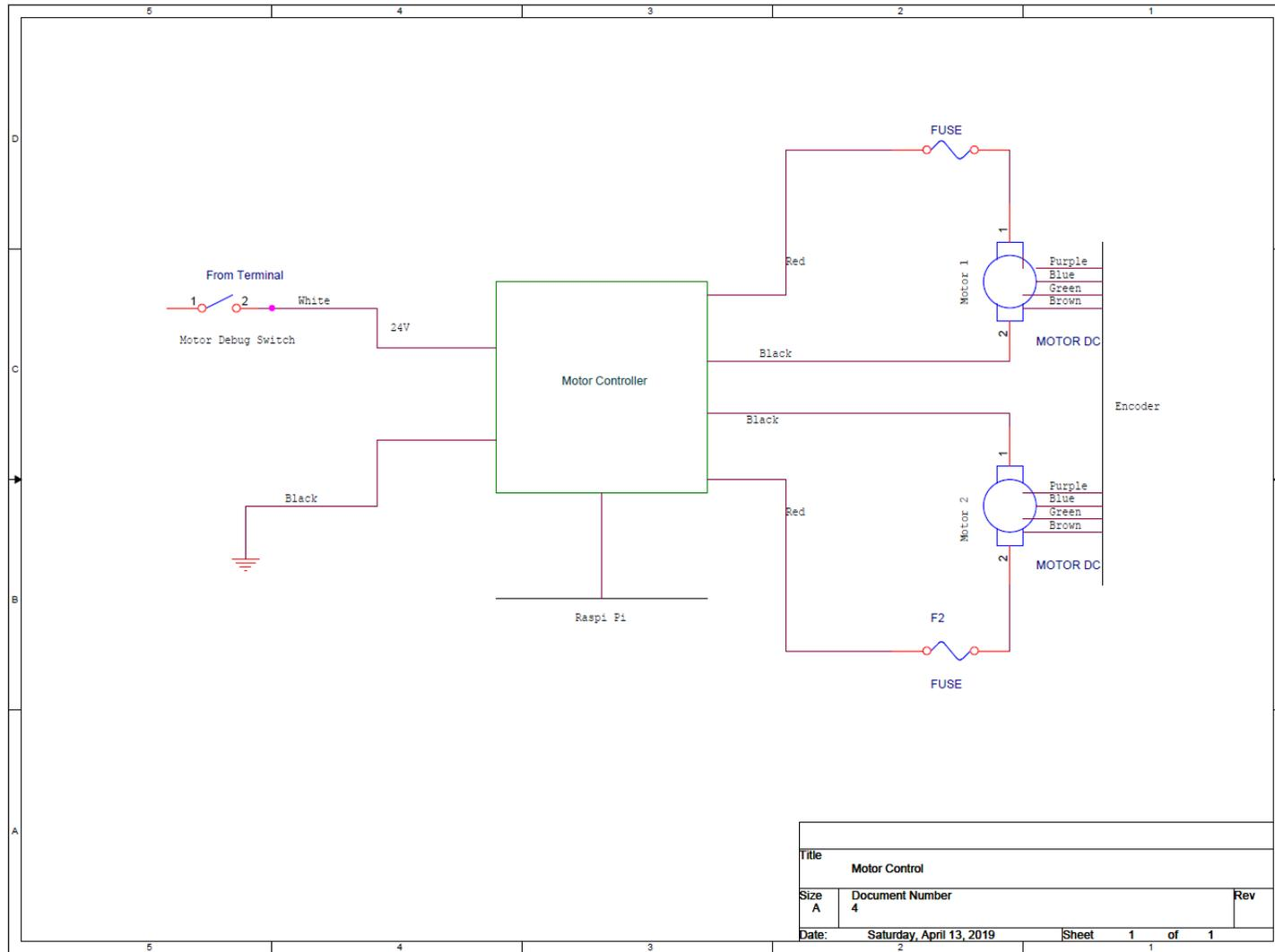
B-6. This schematic demonstrates the robots motor control system with operation of two DC motors with an inline fuse connection.
