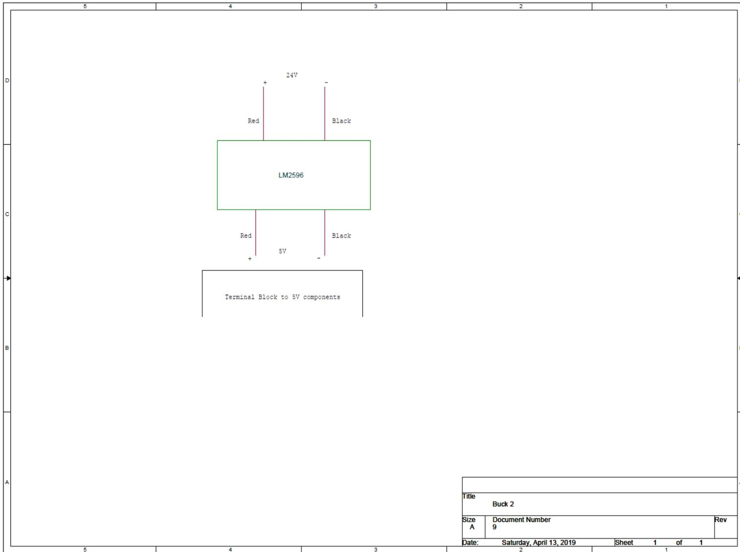
B-2. Wiring diagram schematic of a DC-DC buck converted stepping down 24 volts to a 5-volt terminal for use of the components.
