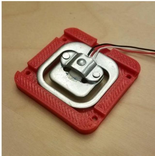
Figure 33. Load Cell Housing [3]
