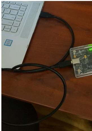
Figure A.26: Connecting BladeRF to Laptop [9]
