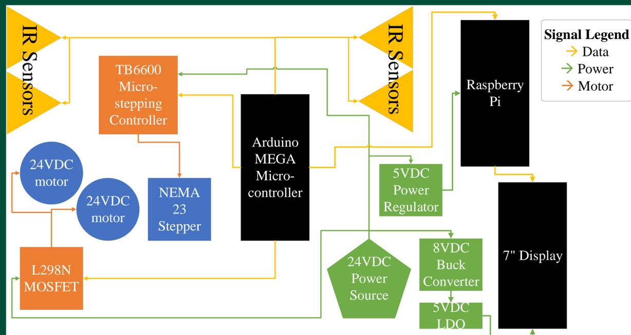
Figure 1: Block diagram of the software and hardware interconnections
