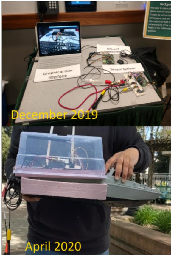
Figure 2: Laboratory Prototype vs. Deployable Prototype [6]
