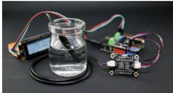
[16] Figure B6: Gravity Analog TDS Sensor
