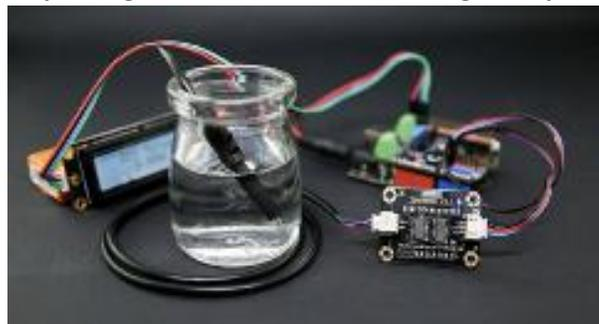
[16] Figure B6: Gravity Analog TDS Sensor
