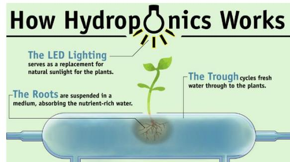
[2] Figure 2: How Hydroponics Works
