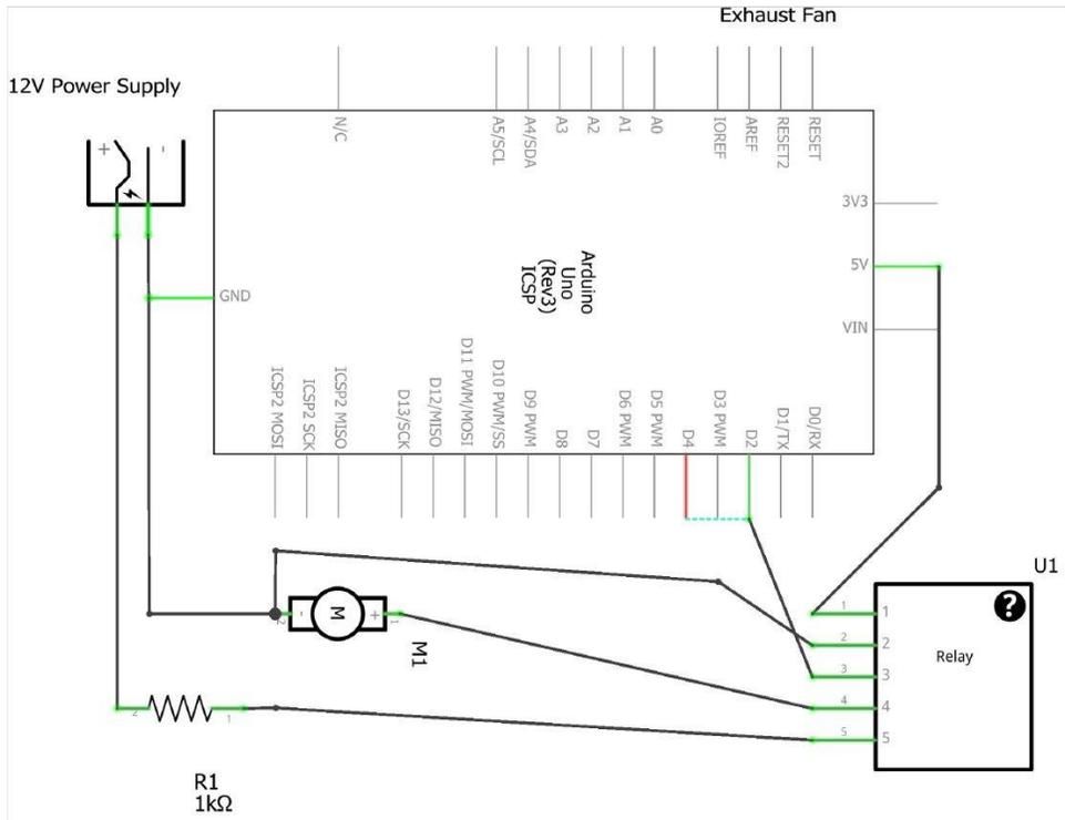
[16] Figure D2. Exhaust Fan Schematic
