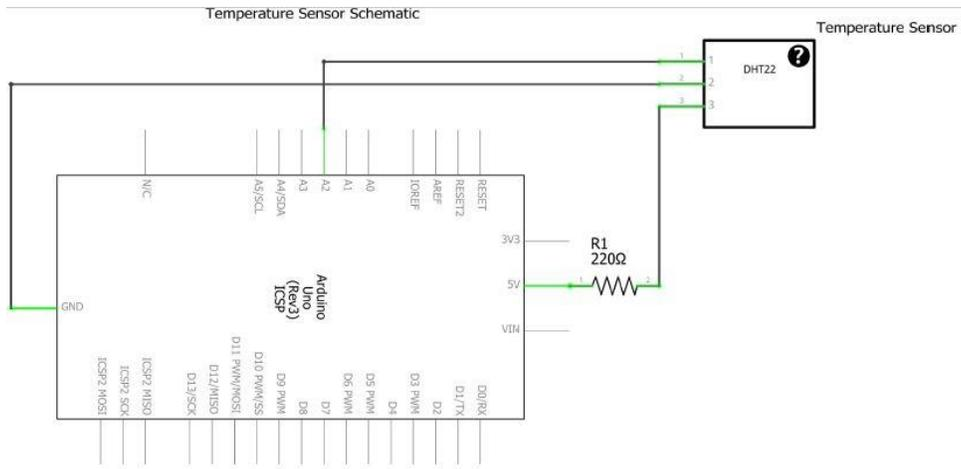
[16] Figure D6. Temperature Sensor Schematic
