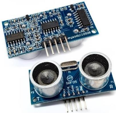
Fig. 33 Ultrasonic sensor [32]
