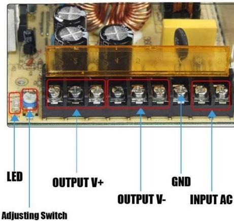
Fig. 43. Power supply's Terminals [40]
