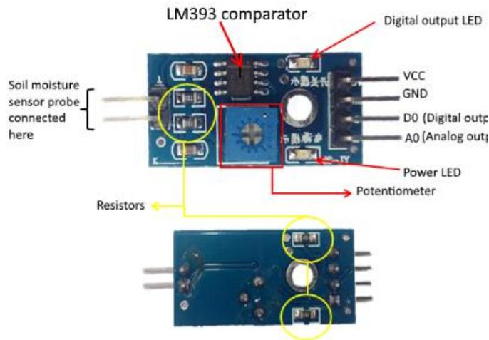
Fig. 9. YL-69 Sensor Components [18]
