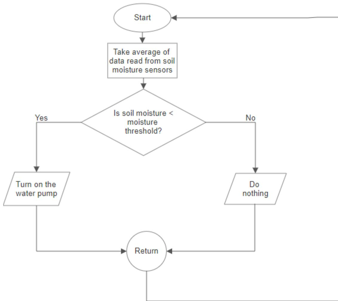
Fig. C4. Logic flowchart for automated soil moisture function [1]
