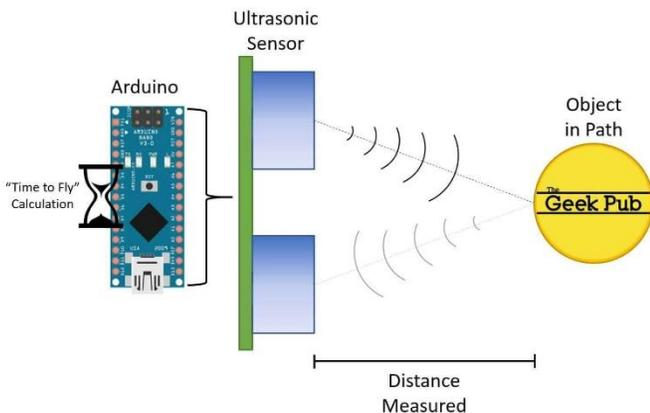
Fig. 34. Ultrasonic Sensor Working Principle [33]
