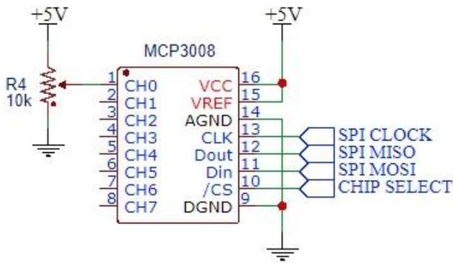
Fig. 12. MCP 3008 ADC Schematic [21]
