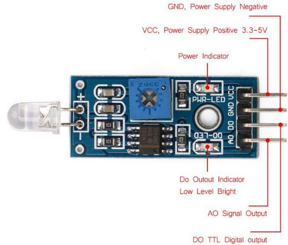
Fig. 10. DROK 200033 Light Level Sensor [19]
