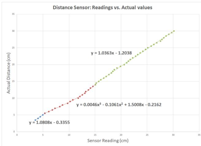
Fig. 51 Water Level Sensors Readings Calibration [1]
