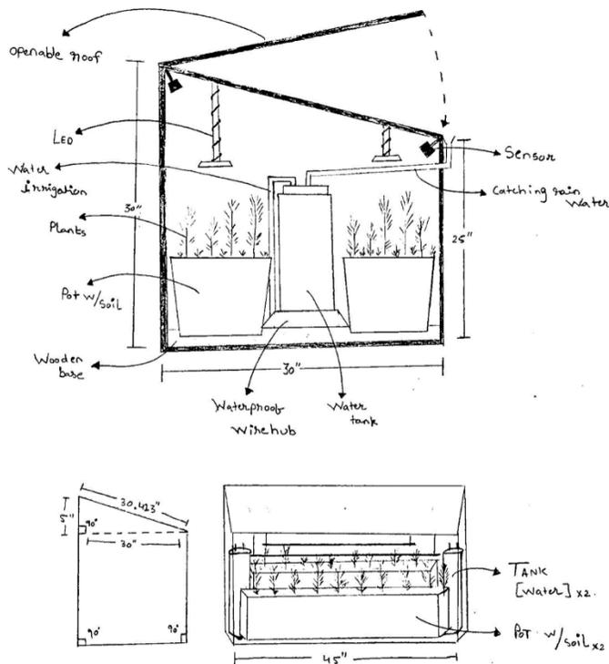
Fig. 62. Conceptual: front & side view of the Smart Greenhouse [1]
