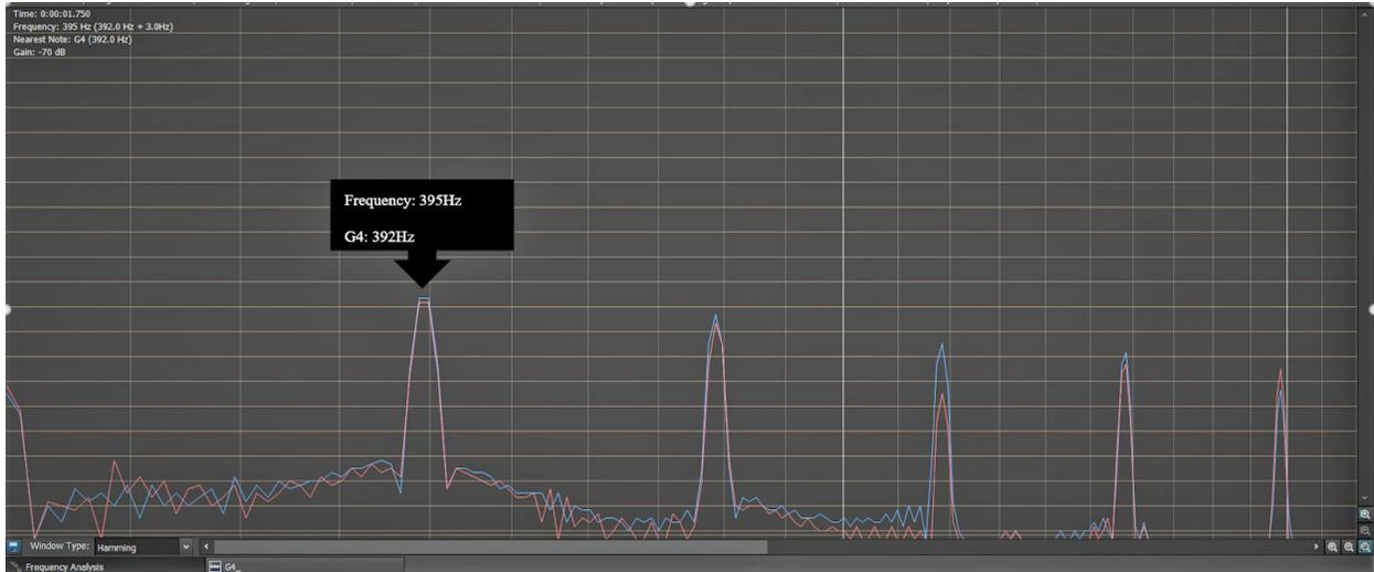
Fig. C5. WavePad G4 Note Gain vs Frequency Waveform [16]
