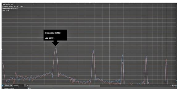
Fig. 3 WavePad G4 Note Gain vs Frequency Waveform [16]
