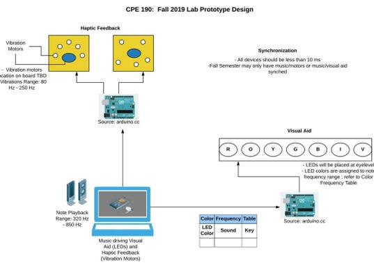
Fig. 1 Fall 2019 Lab Prototype Design Schematic [9]
