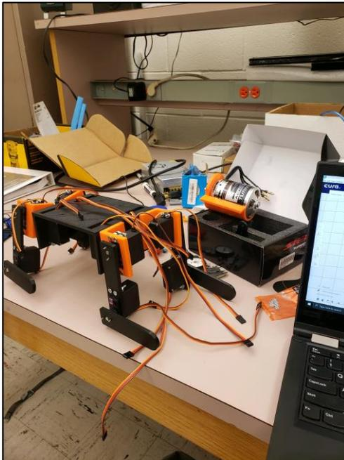
Figure 5.4 3D Printed Small Scale Dog Model
