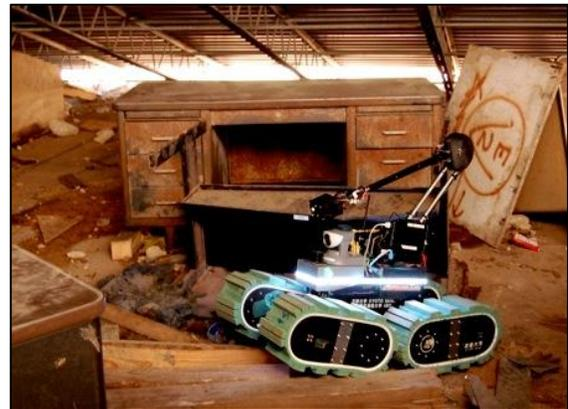
Figure 2.11. KOHGA3 Ground Robot for Search and Rescue and Vacant Building Inspection
