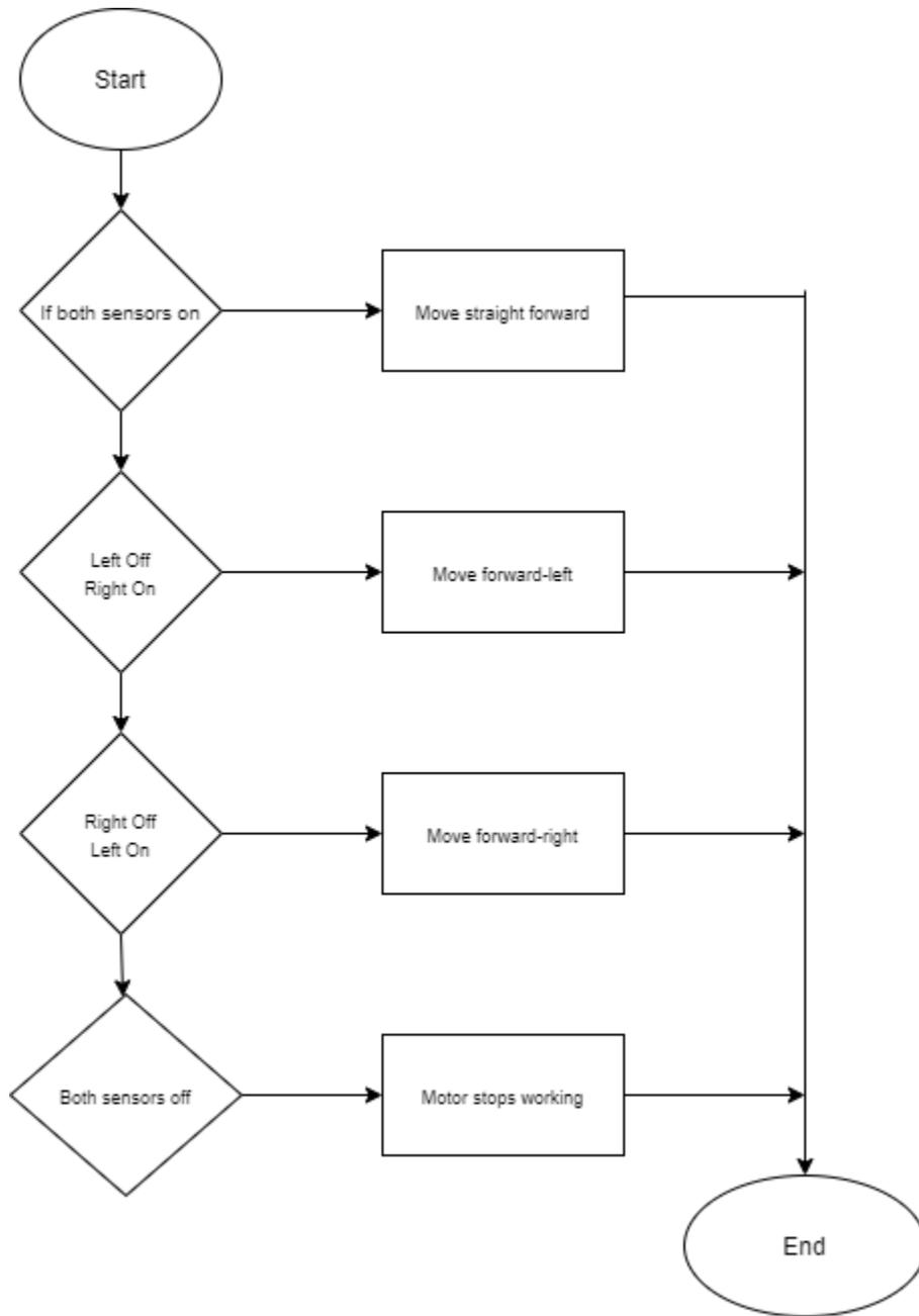
Figure C1: Infrared Sensor Line-following Subroutine
