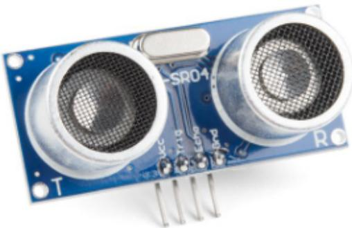
Figure 12. Ultrasonic Sensor
