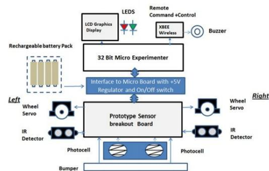
Figure 3 : Layout of autonomous robotS
