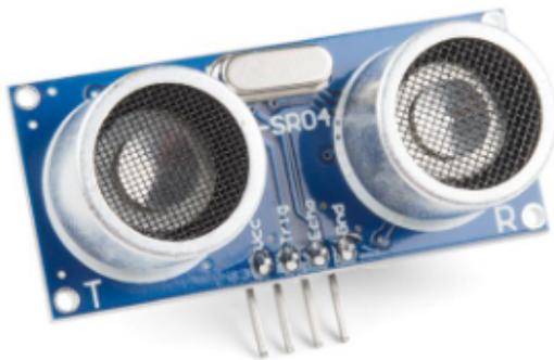
*Figure 23: Ultrasonic Sensor*
