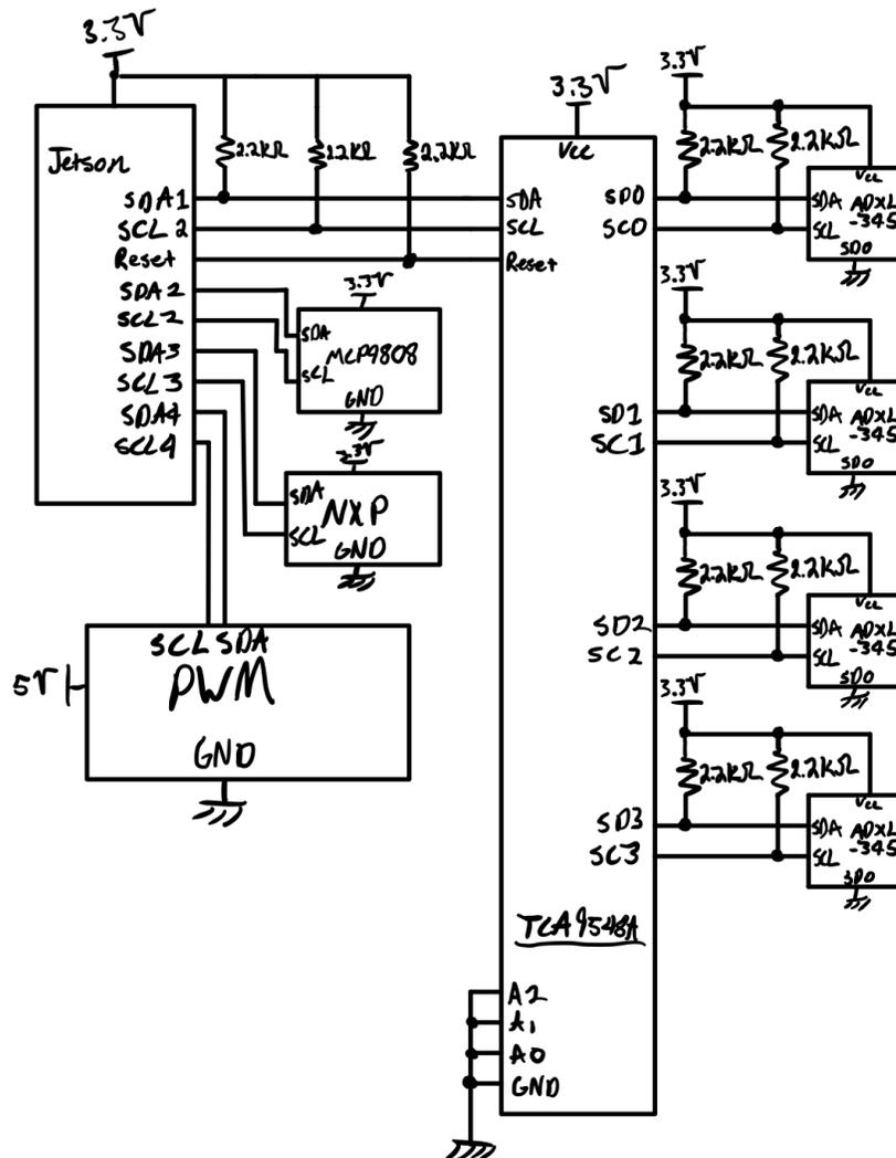
Fig B2. I2C Circuit Schematic [27]
