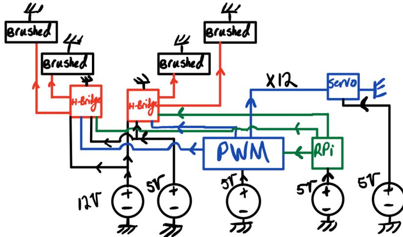
Fig B1. Full Motor Control Circuit Schematic [27]
