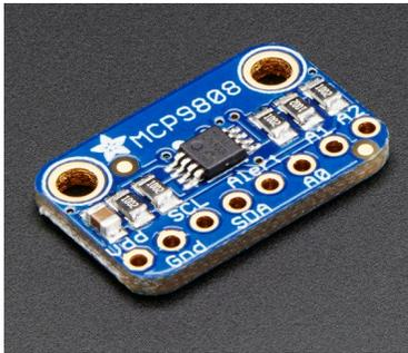
Fig 10. MCP9808 Temperature Sensor [22]
