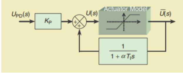
Fig 9. Common PID Controller Schematic [21]
