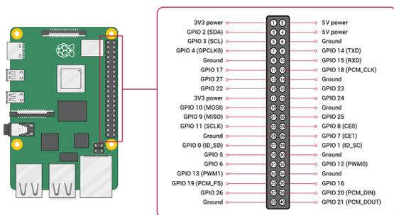
Fig 7. Rpi 4 Pin Layout [19]
