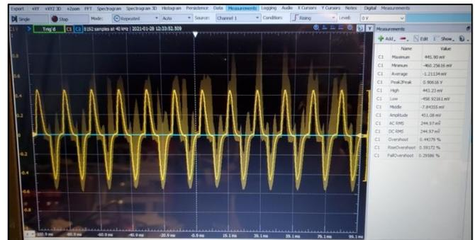
Figure A-29. Ethernet Signal Detection.
