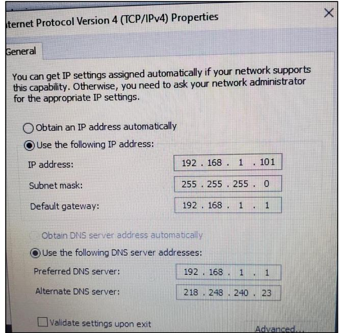
Figure A-44. IPv4 Manually Configured Network properties.
