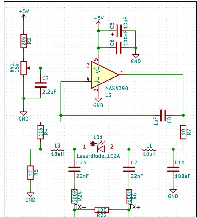
Figure A-15. Transmitter design. [[6] [6]
