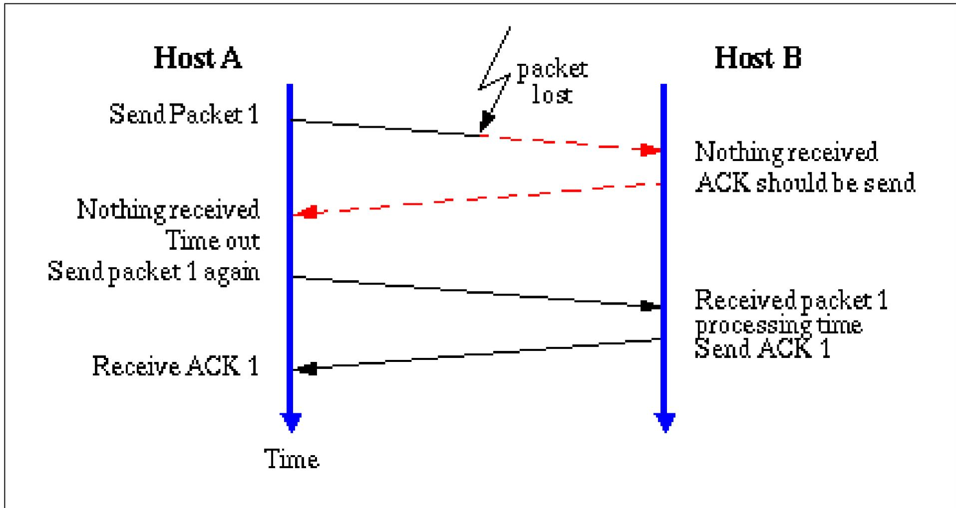
Figure A-10. Data transmission between two devices.
