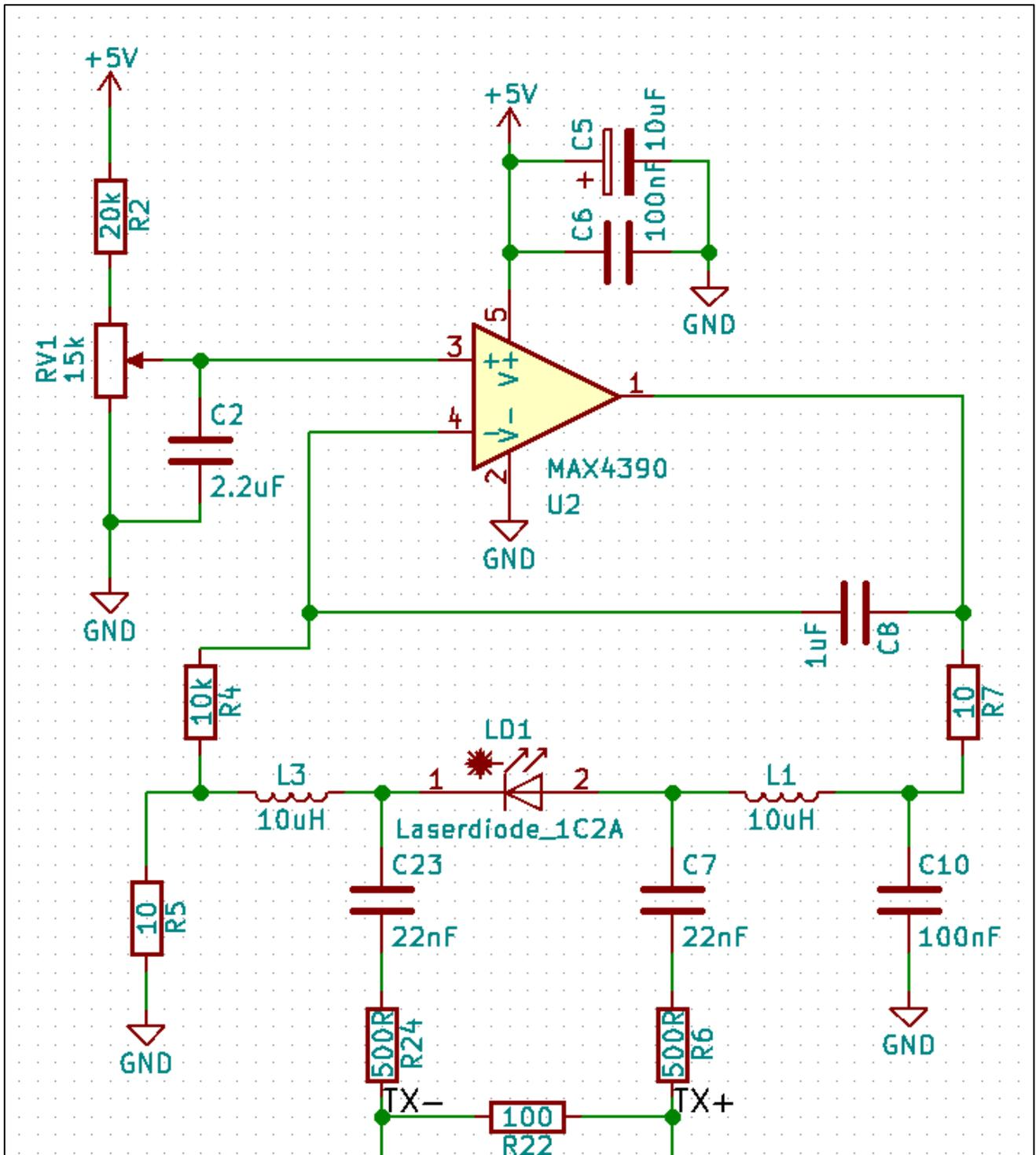
Figure A-15. Transmitter design. [[6]]
