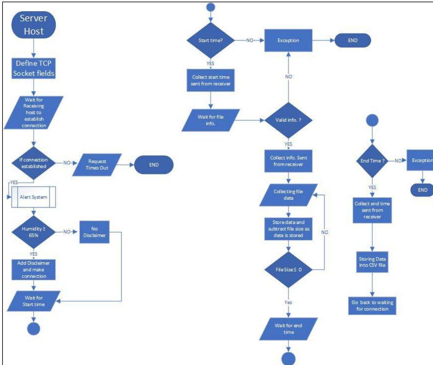
Figure D- 1. Server Socket Flow Chart
