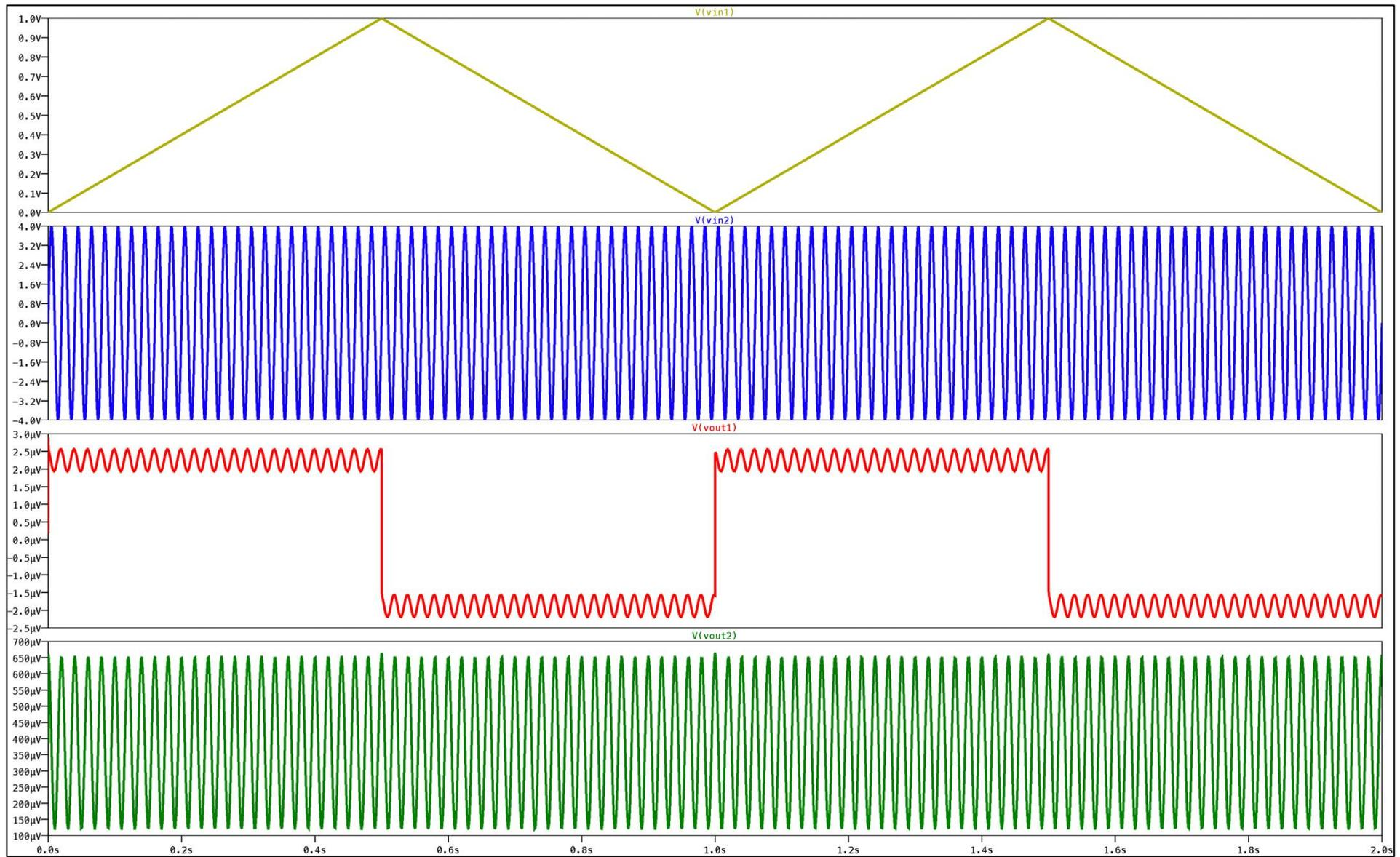
Figure A-18. Results of the MAX4390 simulation.
