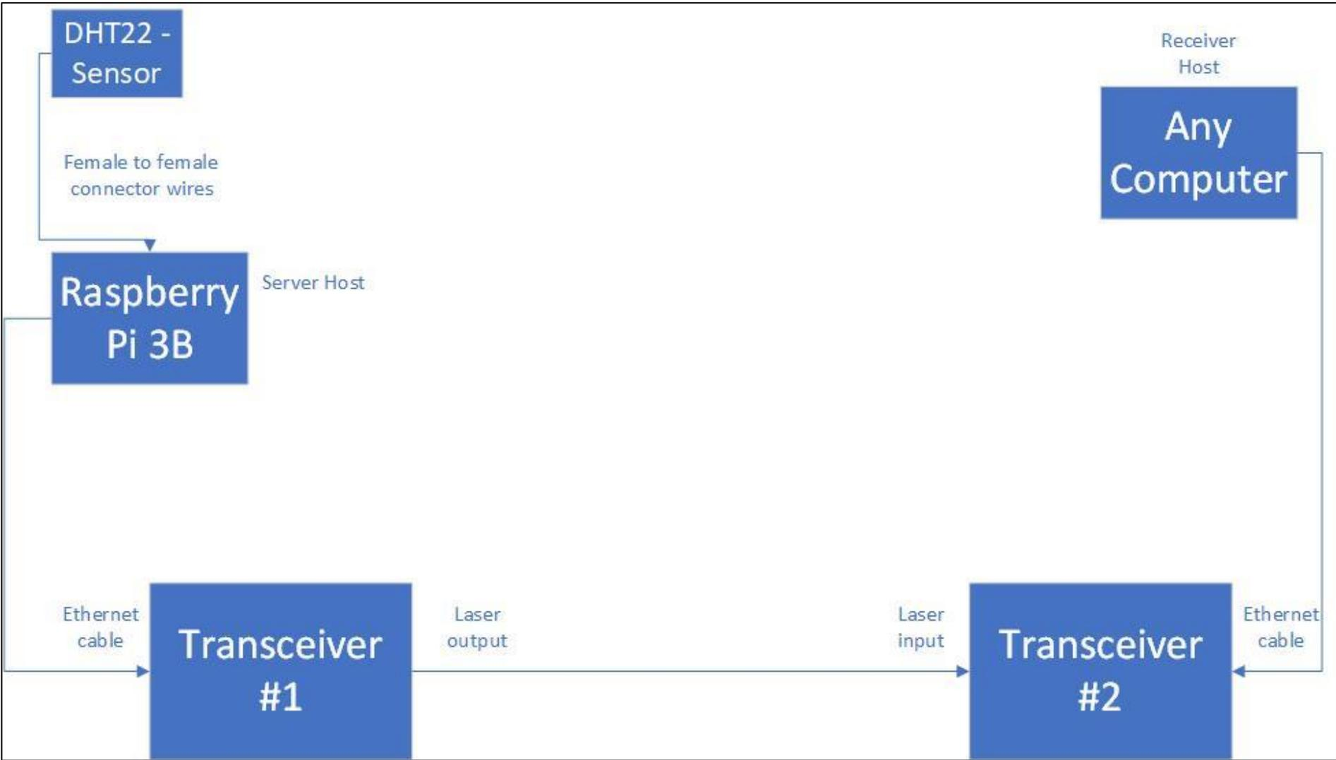
Figure C- 1. Hardware Block Diagram
