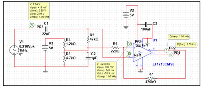
Figure A-22. LT1713 Op-amp design on Multisim.
