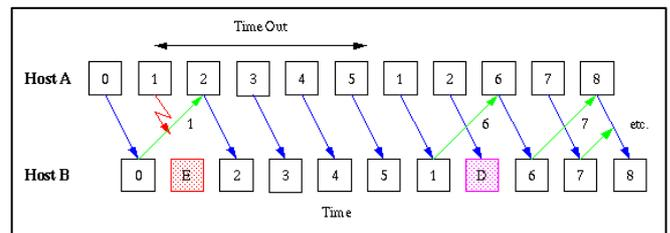
Figure A-11. Data transmission between two hosts. [25]
