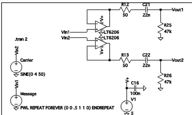
Figure A-25. MAX4392 Shown with Test Message and Carrier Signals.
