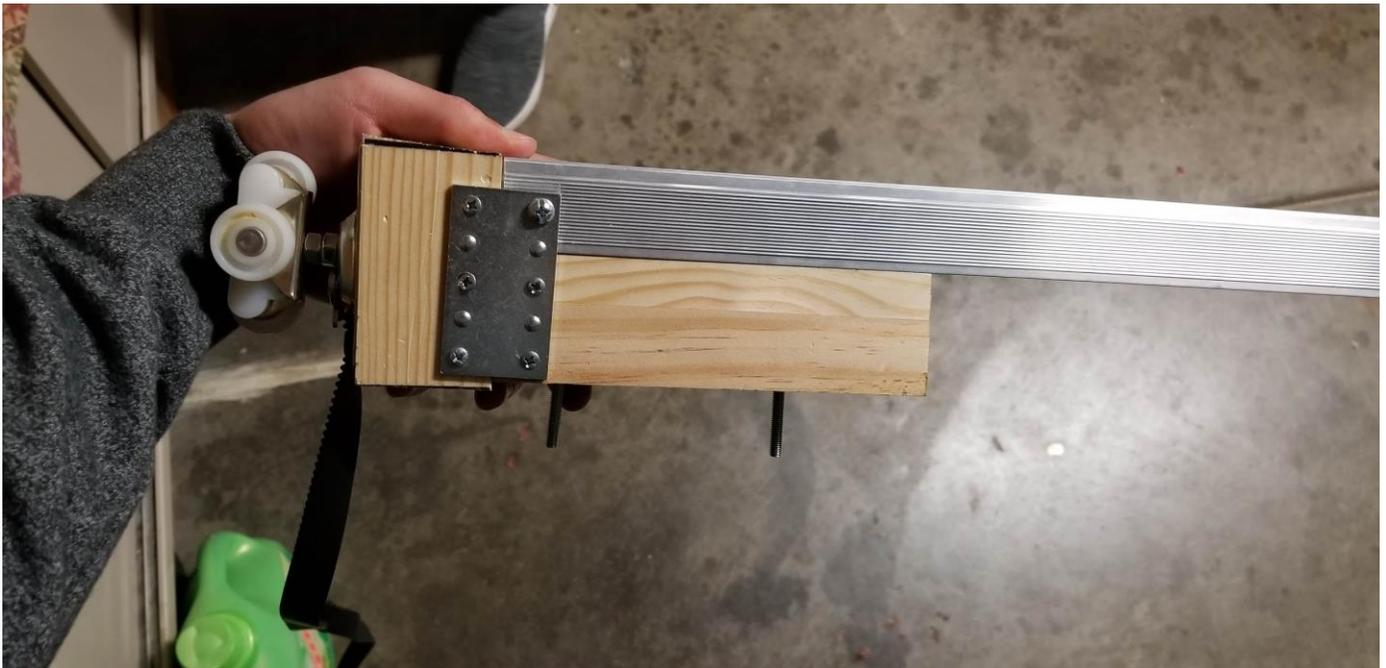
*Figure D 6: Mount used to hold Horizontal slider with Vertical slider [52]*
