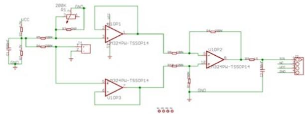
Figure 16. GSR amplification circuit [32]
