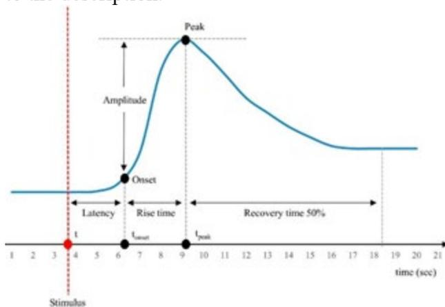
*Figure 12. Example of GSR spike and components of the curve used in determining magnitude of stress response [32]*
