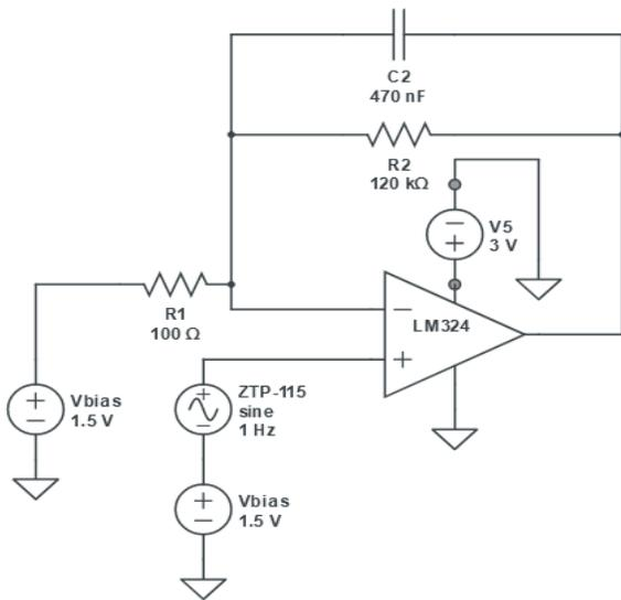
Figure 13. Temperature Sensor Amplification Circuitry [30]
