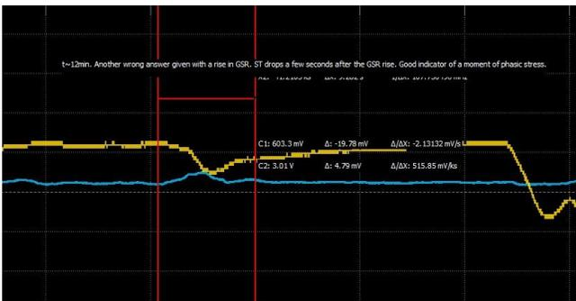
Figure 14. GSR measurements (Yellow) vs Skin Temp. (Blue). The area between the red lines indicates the introduction of a stressor, resulting in the following spikes and dips in the respective waveforms [30]
