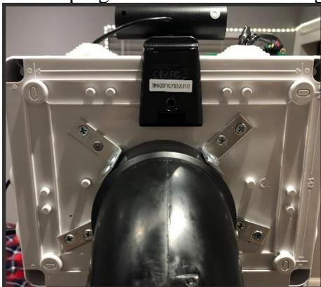
Figure 51: Back of case with case braces [17]
