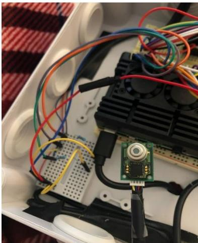
Figure 25: D6T-32L Temperature Sensor [17]
