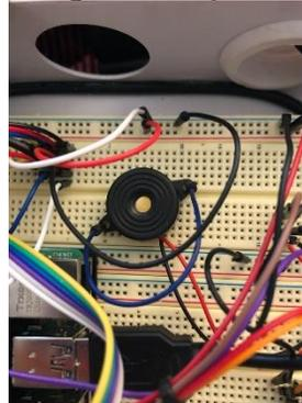
Figure 31: Piezo buzzer [17]
