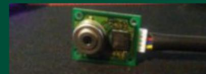
Figure 2: D6-32L Infrared Sensor [2]
