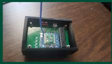
Figure 1: Wearable Tag with Casing
