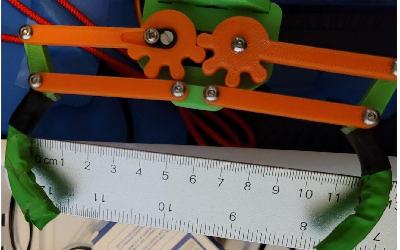
**Figure D9.** New +22mm (lengthwise) Extended Grip Parts to get outer width of ~11cm and minimum opening of ~10cm printed in Orange Hatchbox PLA and Green 3DSolutech PLA. [57]
