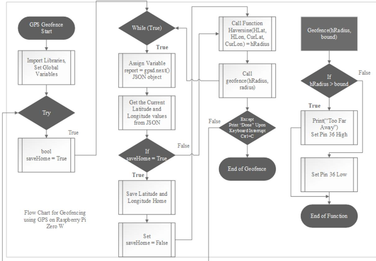
**Figure C1.** GPS Geofencing FlowChart/Pseudocode [56]
