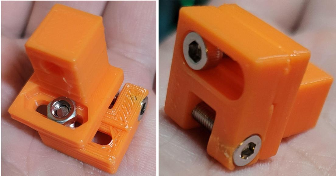
**Figure D11.** Camera Case Mount with Sliding Functionality [57]
