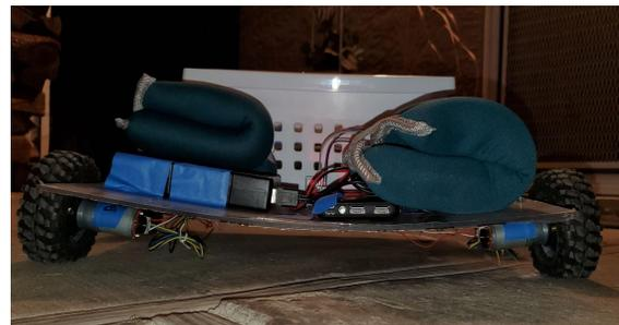
FIGURE 15 - “BASE IMMOBILE AND BENDING AFTER 12LB WEIGHTS ADDED ” [32]
