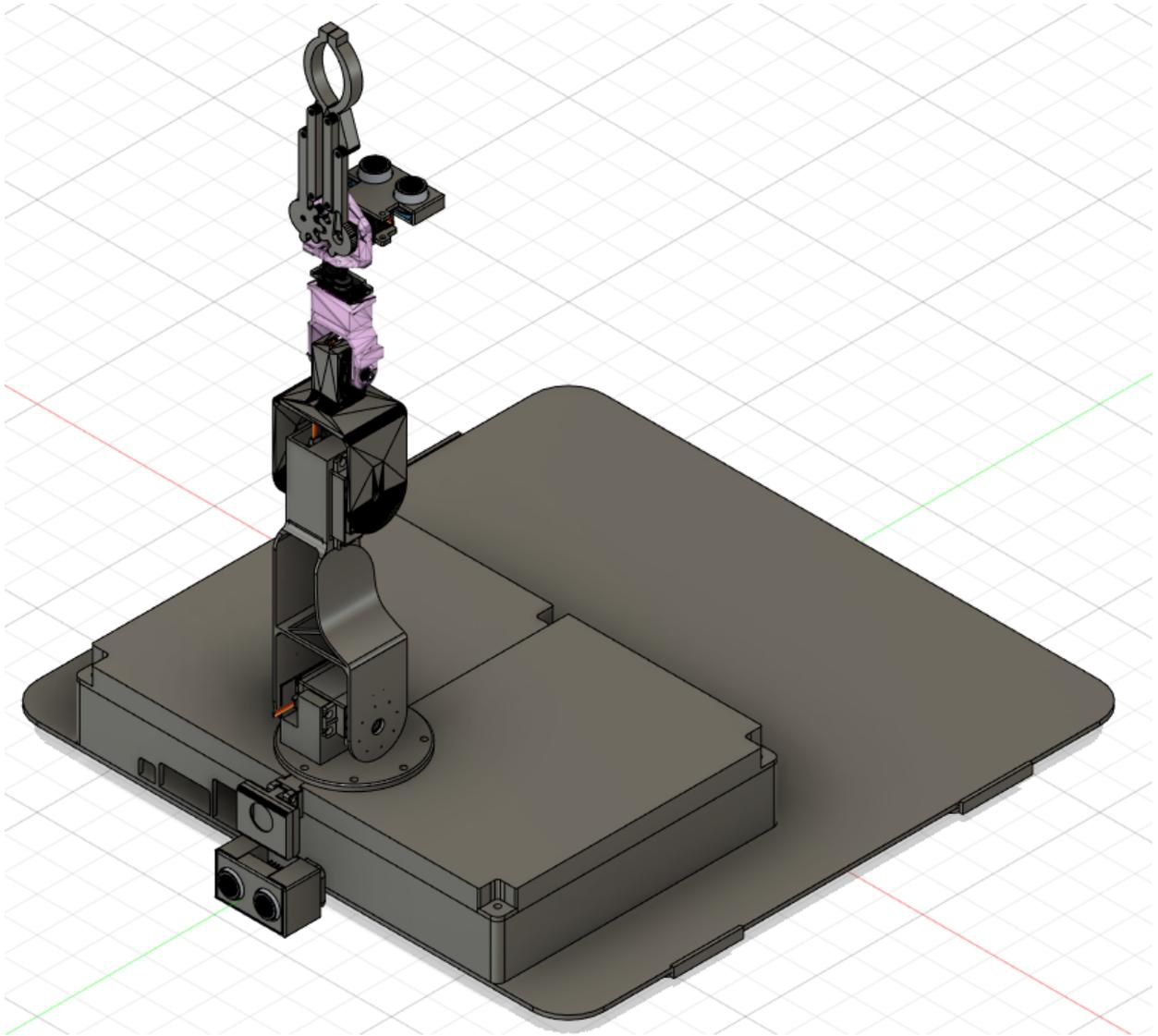
**Figure D5.** 3D CAD Incomplete Chassis with Arm and Sensors [57] Parts seen in pink are borrowed from user named holgero from Thingiverse [58] while the rest are a remix for our use case. Big servo adapter [59] Small Servos adapter [60] Sonar sensor casing [61].
