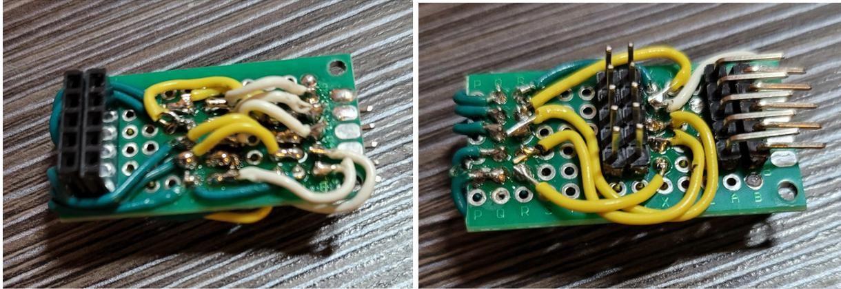
**Figure B1.** Protoboard I2C Bus Extension for use with the Adafruit Servo Hat and Berry GPS-IMU (Unused) [47]
