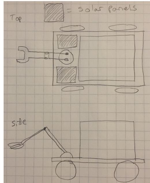
FIGURE 9 - EARLY LAB PROTOTYPE SKETCH OF A LITTER BOT DESIGN [25]
