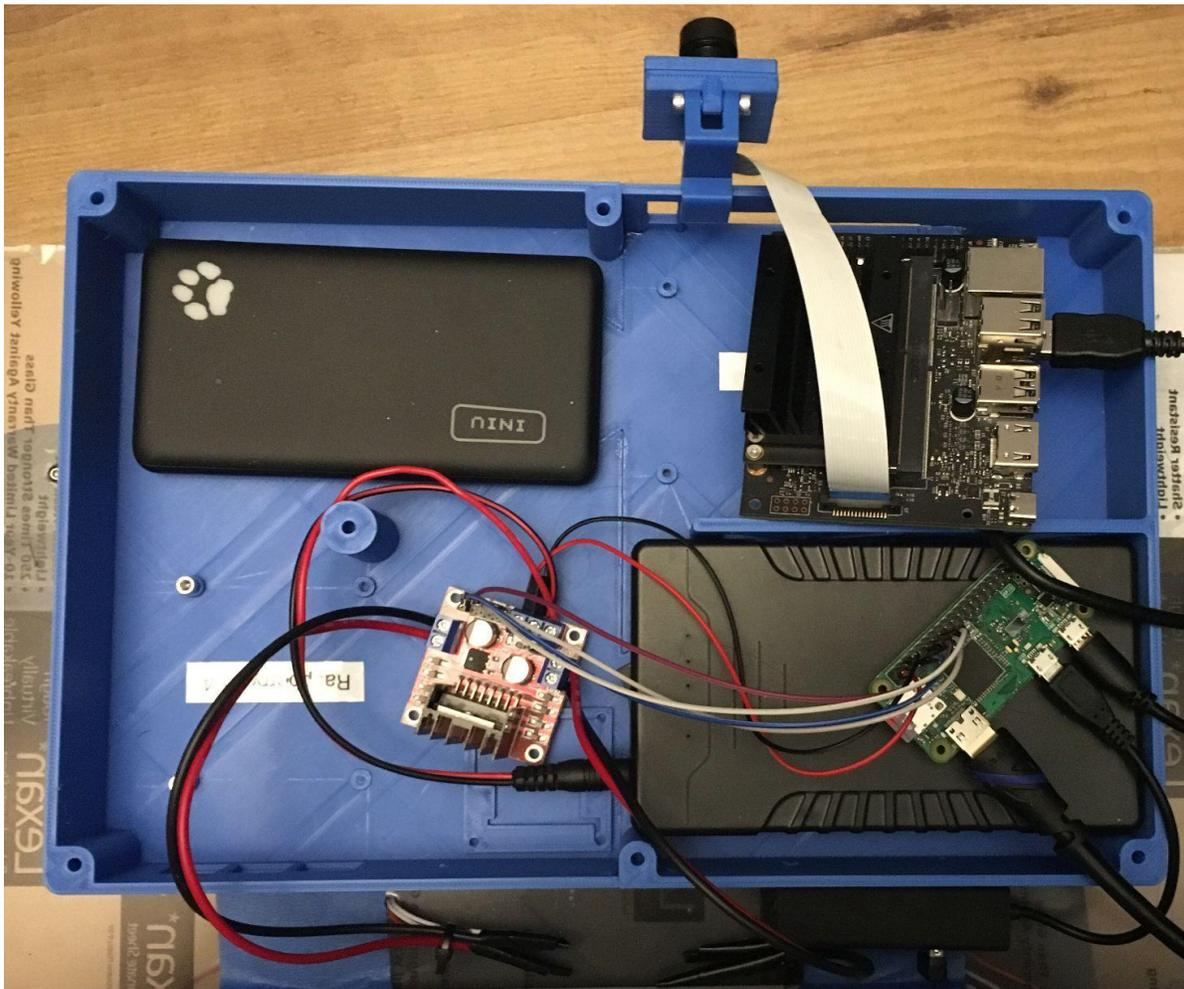
**Figure D7.** Initial Components Mockup with Temporary Camera Mount [57]
