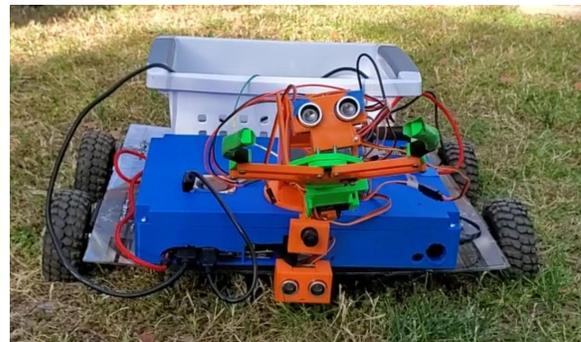
**FIGURE 28 -** DISTANCE SENSORS AND FRONT VIEW OF LITTER BOT [27]
