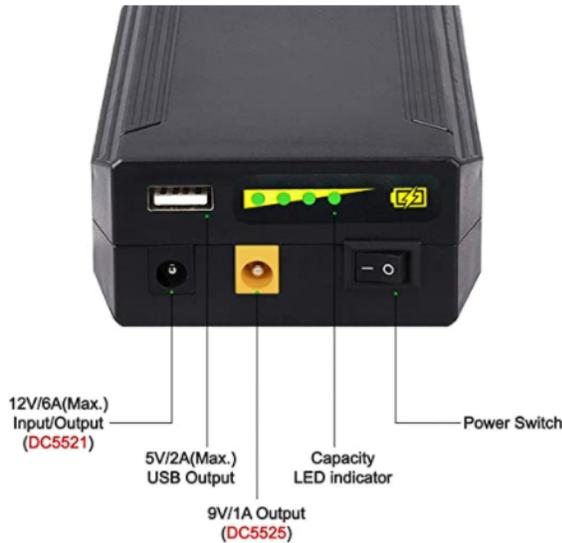
FIGURE 16 - “TALENTCELL MULTI-OUTPUT LI-ION BATTERY” [33]
