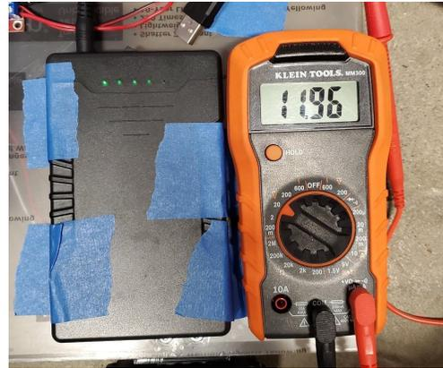
FIGURE 19 - “MEASURING THE VOLTAGE OF 12V BATTERY AT 80% CHARGE” [36]
