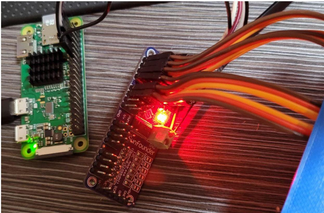
**Figure B2.** Raspberry Pi Zero W with Sunfounder Servo Hat connected via I2C [47]
