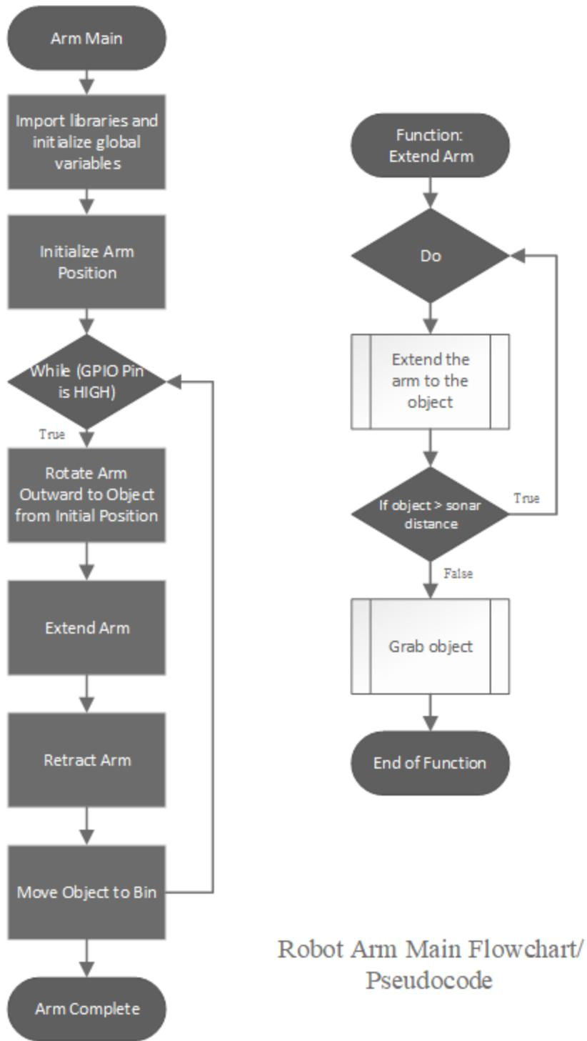
**Figure C3.** Robot Arm Flowchart/Pseudocode [56]
