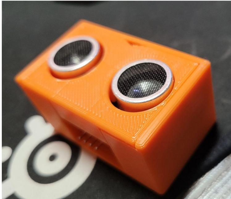
**Figure D10.** HC-SR04 Sonar Sensor in Orange Hatchbox PLA Case [57]
