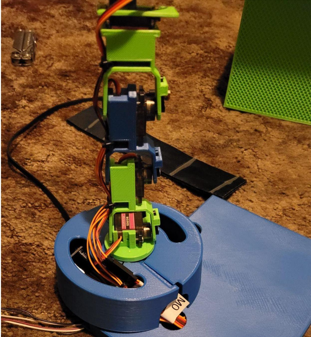
**Figure D17.** Second Arm with Stabilizer and tight cable management [57]
