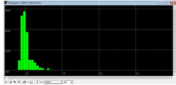
**Figure 21.** Histogram of the HDOP (Horizontal Dilution of Precision) (Inside) [39]
