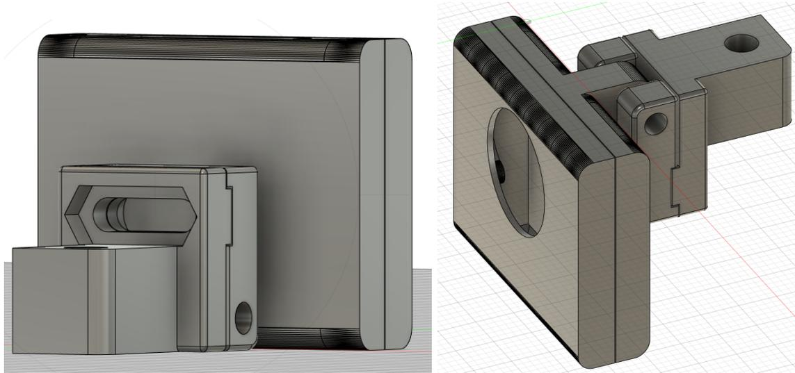
**Figure D15.** Camera Case and Mount Rear (Left) and Front (Right) [57]
