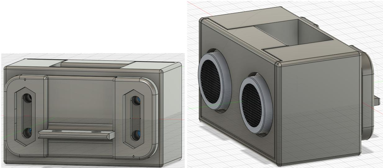
**Figure D16.** Front Center Mounted Sonar Rear (Left) Front (Right) [57]
