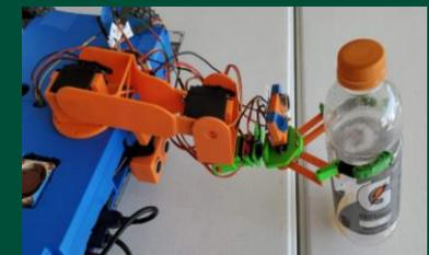
Figure 5: Gripper Arm.
