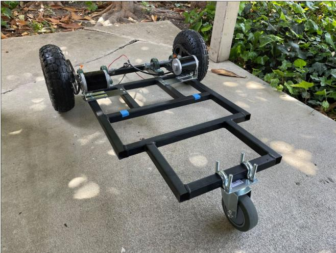
Figure 19. Deployable Prototype Welded Steel Frame.
