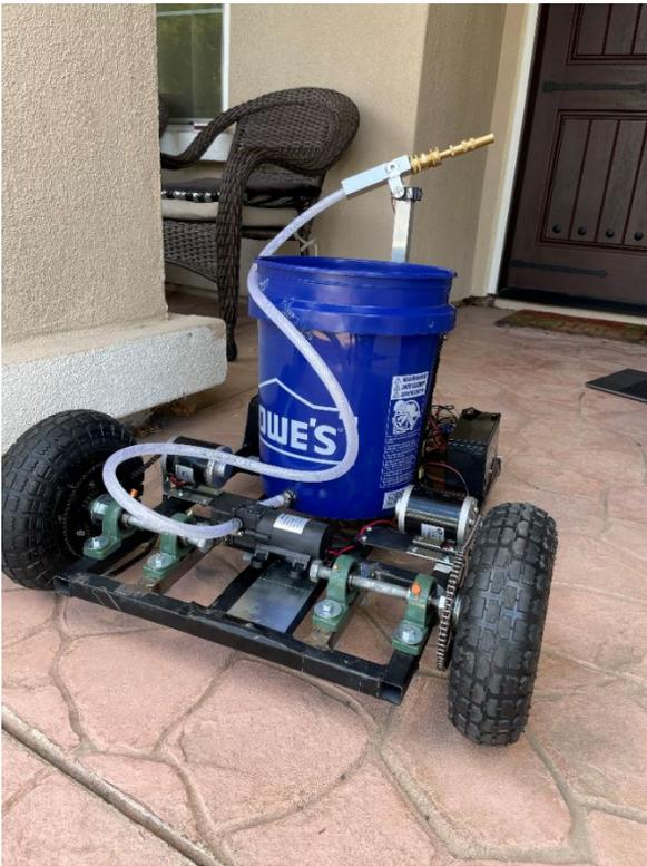
Figure 16. Spray Nozzle Hose Assembly.
