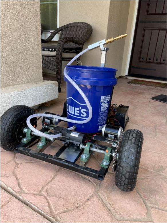
Figure 22. Spray Nozzle Hose Assembly.
