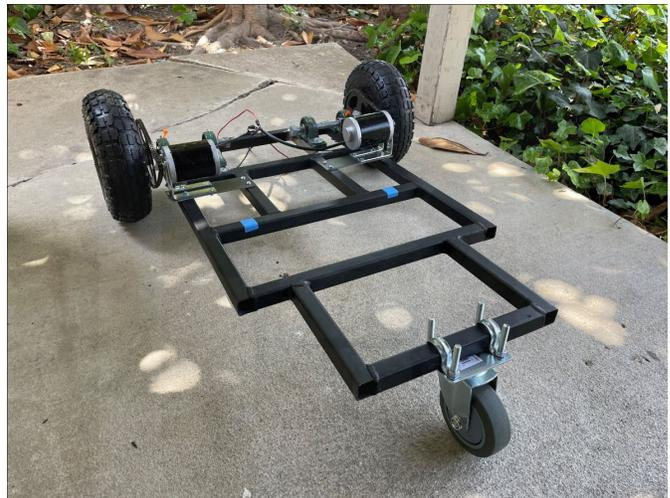
Figure 13. Deployable Prototype Welded Steel Frame.
