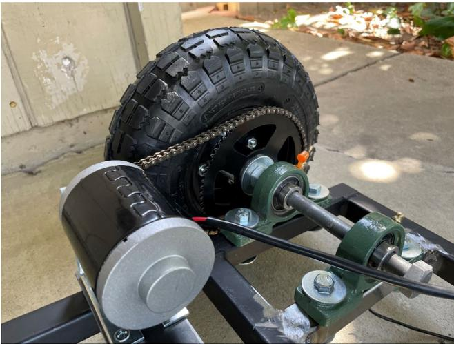
Figure 20. Deployable Prototype Welded Steel Frame.
