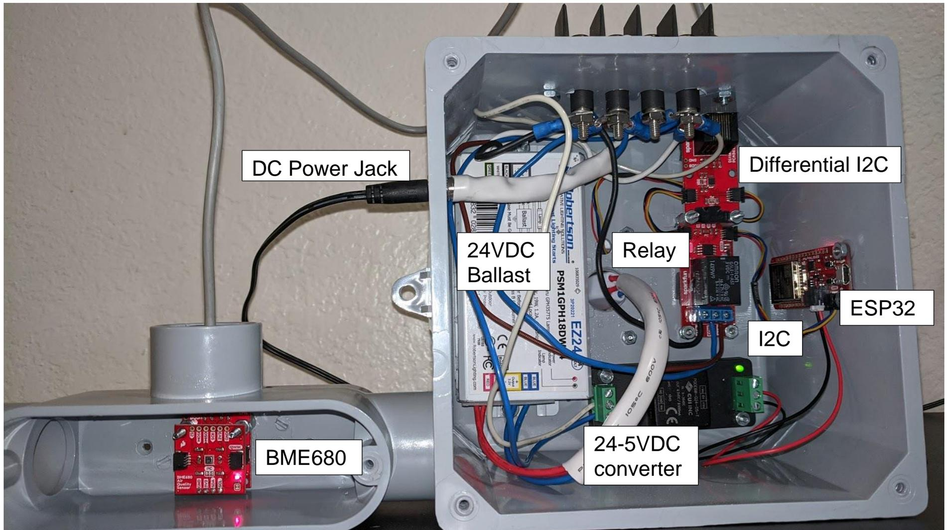
Figure B-3 Inside Prototype Hardware [30]
