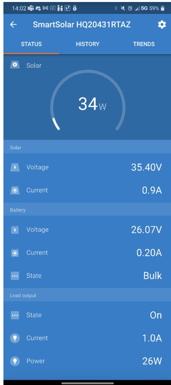
Figure IX-6 2pm MPPT Power status for the panel, the battery, and the system current and wattage. [37]
