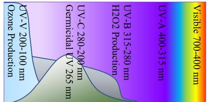
Figure II-1 UV light spectrum [3].
