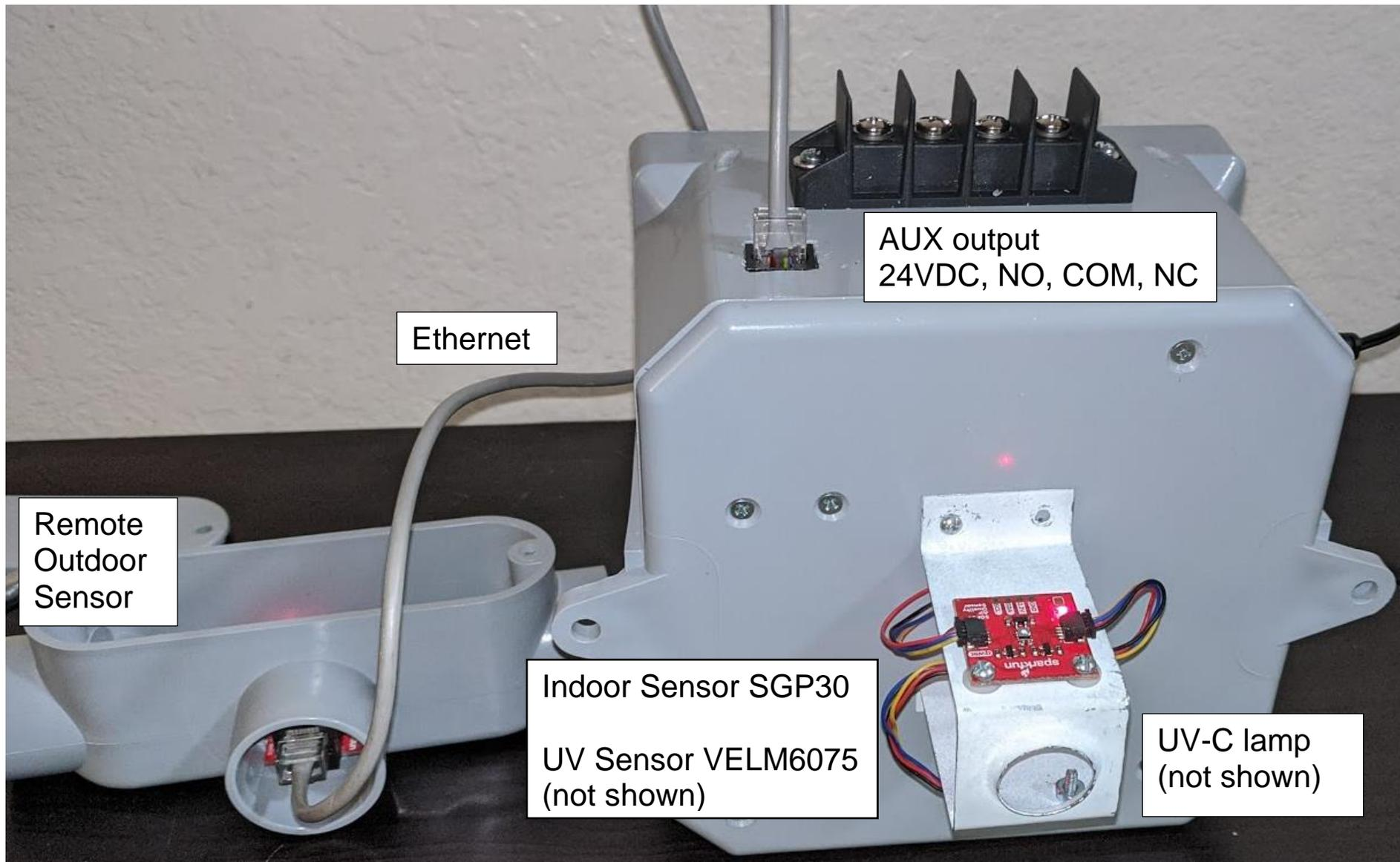
Figure B-4 Outside Prototype Hardware [30]
