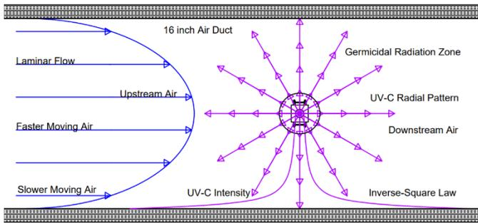
Figure IX-2 Laminar Flow Germicidal UV Dosage [27]
