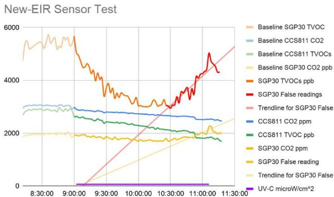
Figure IX-3 TVOCs lower by UV-C [27]
