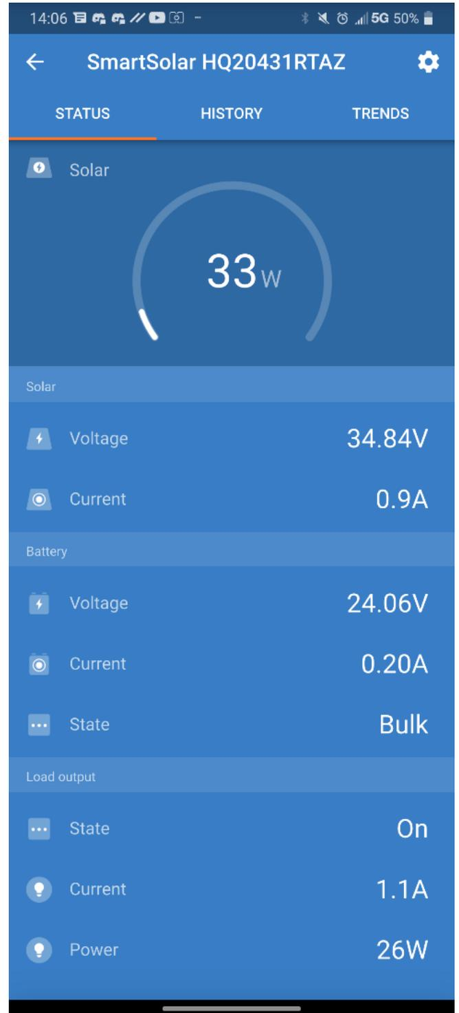
Figure IX-7 The 7am MPPT status for the panels, batteries, and system current and wattage [37]
