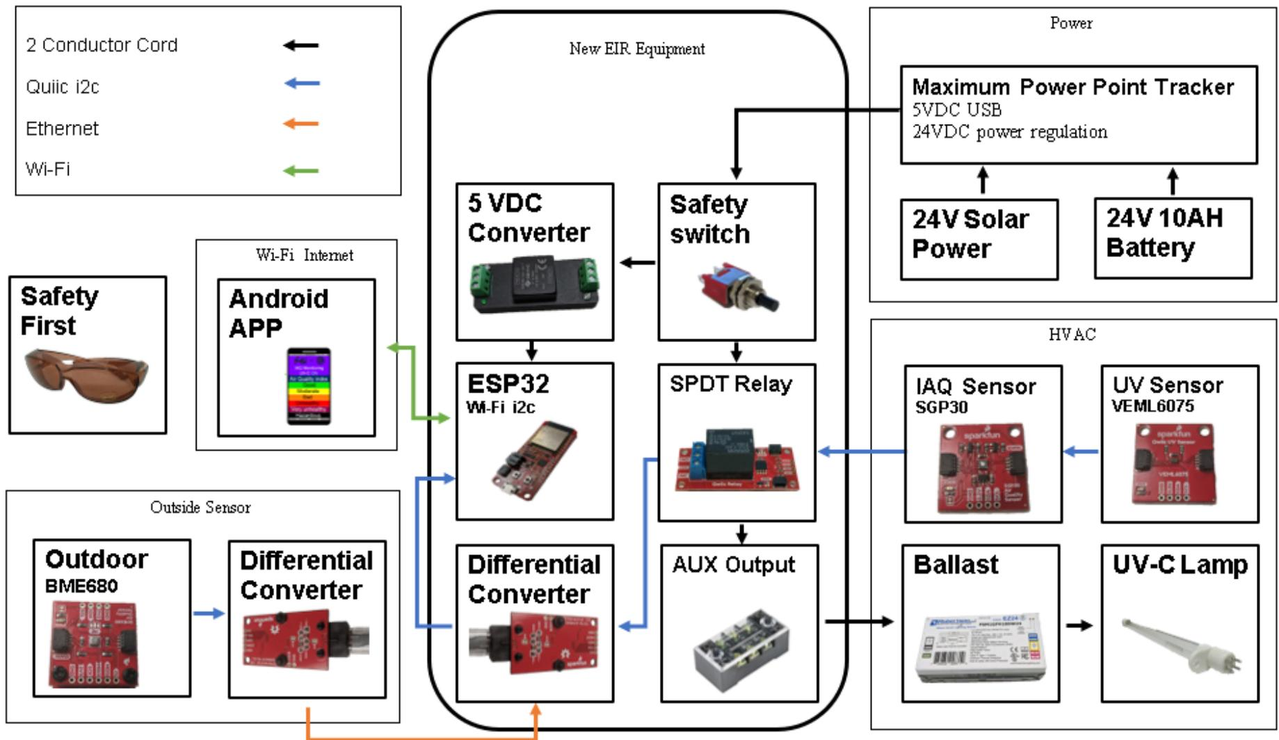
Figure B -3 New-EIR Hardware Connections[30]
