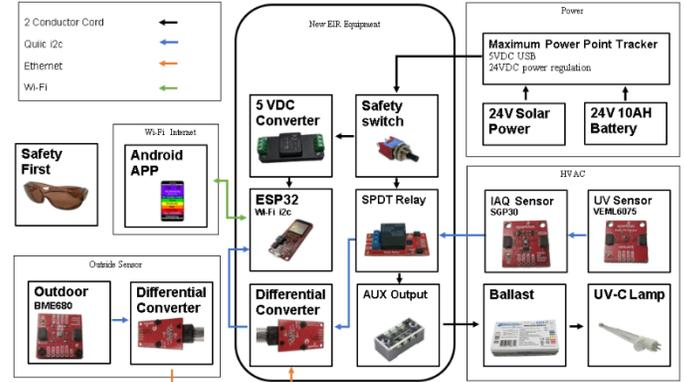
Figure III-2 Hardware Connection [29]
