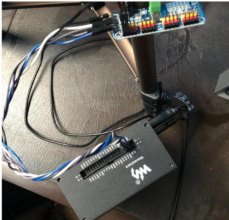
Fig. C2. Servo Driver Connected to Jetson Nano [43]
