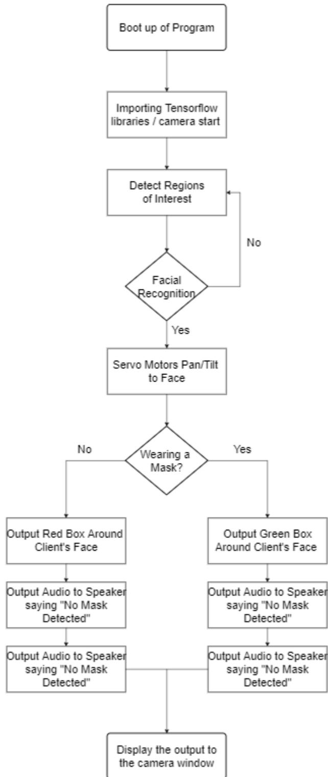
Fig. B1. AI Algorithm Flowchart [39]
