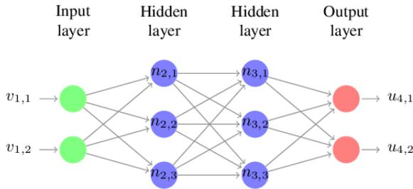
Fig. 8. Simple neural network where “n” represents the dependent nodes that receive the input from the input layer and processes it, creating a classification that is then passed to the next hidden layer [9]
