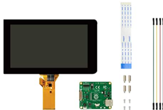
Figure 12. Raspberry pi Touch Screen Display [31]
