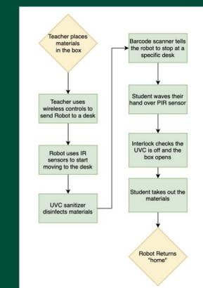
Figure 3: Example Flowchart of Robot's Functionality
