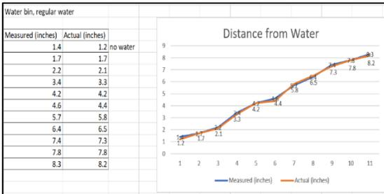
Figure 13: Water level test. Test results and screenshot by Team 8 [11].
