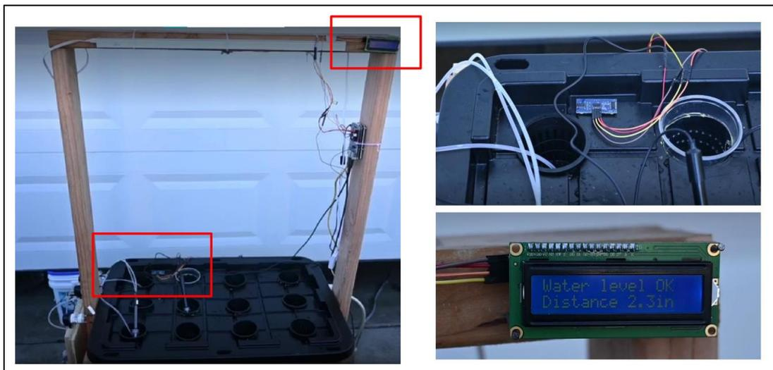
Figure A2: Water Level Sensor Integration [12]
