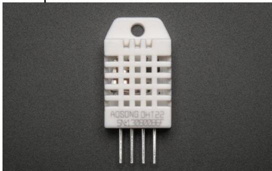
Figure 12: Temperature and Humidity Sensor [13]
