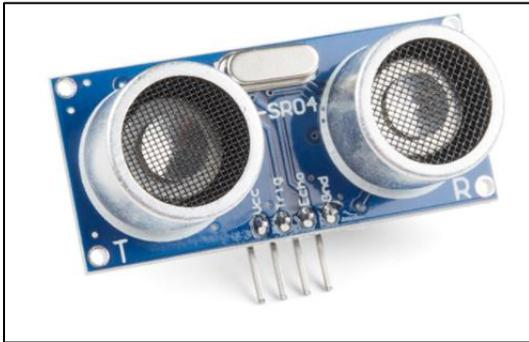
Figure 7: HC-SR04 Ultrasonic Module Distance Sensor; photo from Adafruit, a product manufacturer and distributor [10]
