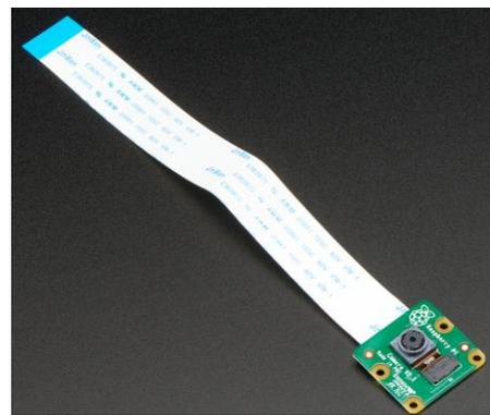
Figure 6: Raspberry Pi Camera Module 2 [13]
