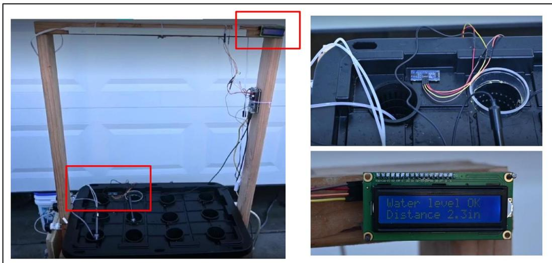
Figure A2: Water Level Sensor Integration [12]
