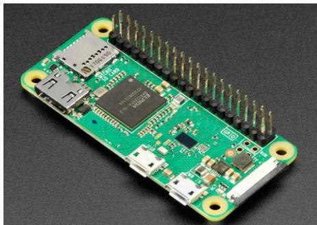
Figure 5: Raspberry Pi Zero W [13]
