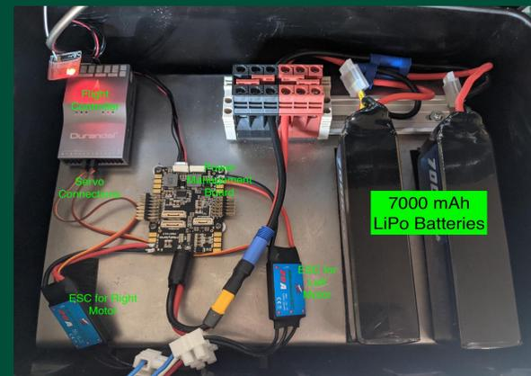
Figure 2: Hardware and Electrical Components
