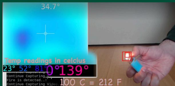
The Above picture shows the flame detection system.
