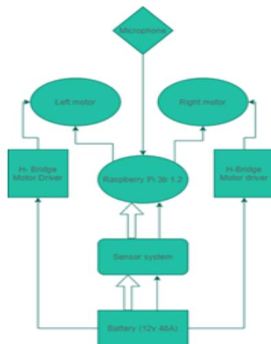
Figure 6 - Flowchart of control system design. Designed using app.diagrams.net
